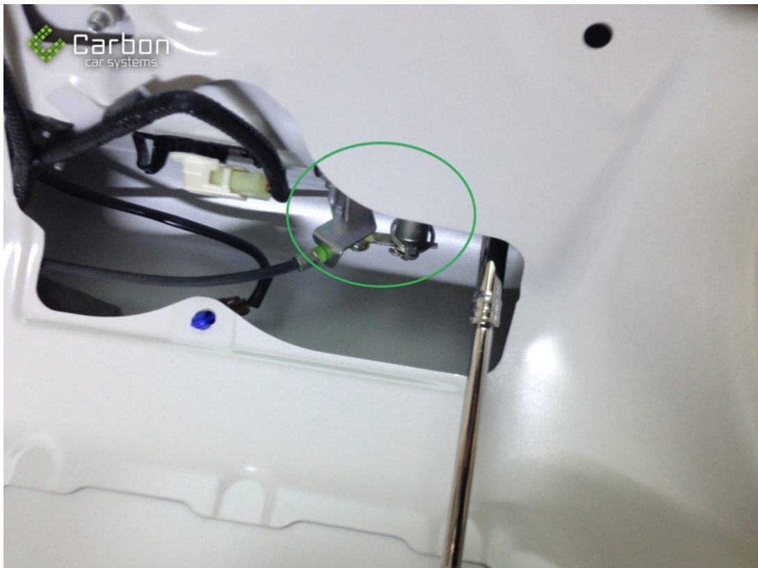
Remove the boot key barrel from inside of lid. Secure this careful so as not to scratch the boot lid.
